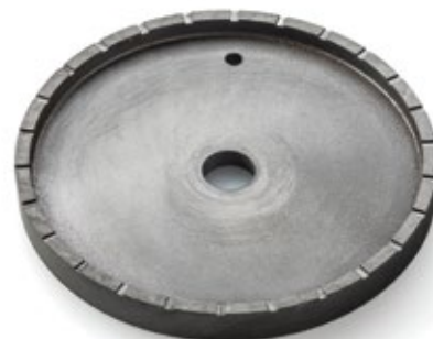
Figure 8.10: Thrustwasher test specimen with lubrication grooves
