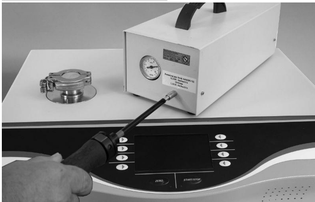
Fig. 17: Sniff test on an external calibration leak
