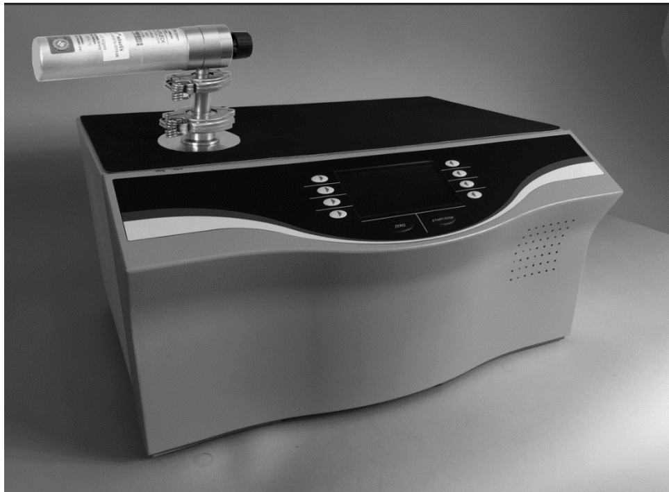
Fig. 15: Checking an external calibration leak
